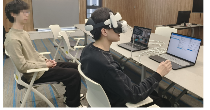
Figure 10: Study 2 apparatus and setup. Right: web interface (MAS) or Guideline Generation page for MAVIS. Left: MAVIS with Meta Quest 3 via wired PC streaming. A facilitator monitored a preview; audio and screen outputs were recorded.
